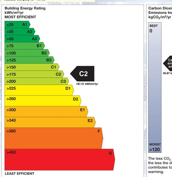
Carbon Dioxide (CO<sub>2</sub>) **Emissions Indicator** Calculated annual CO<sub>2</sub> emissions 36.87 kgCO<sub>2</sub>/m<sup>2</sup>/yr The less CO<sub>2</sub> produced, the less the dwelling contributes to global
